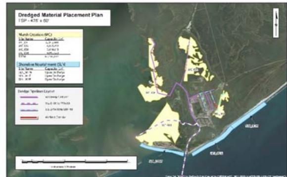
GIS performed hydro-survey and hydro-dynamic modeling as part of the study to determine volumes for approximately 6 miles of channel dredging. GIS prepared the Dredge Material Management and Disposal plans for over 23 Million Cubic Yards of construction dredge material and 63 Million Cubic Yards of 50-year maintenance dredging, all used for wetland restoration and beach nourishment.
