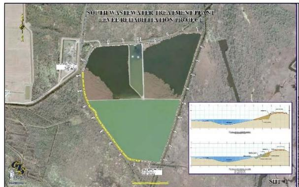
GIS prepared plans to stabilize and restore the original cross-section of the levee and evaluated revetment alternatives for protection and prepared cost analysis for each alternative.
