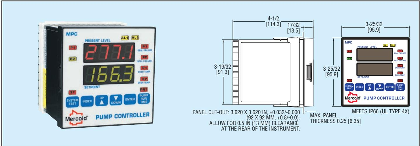
The Mercoïd® MPC Pump Controller provides versatile level control in a standard 1/4 DIN package. Designed for use with almost any style level transmitter the unit displays the present level and main set point value. Incorporated in the MPC is programmable level differential for on/off control of one or two pumps, valves, or other devices through two SPDT relays. Also featured are two additional programmable alarm contacts with front alarm light indication.
