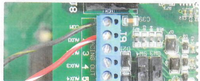
AUX1 and COM connected to external switch
