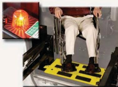
Hydraulic roll stop engages and locks before the platform leaves the ground
