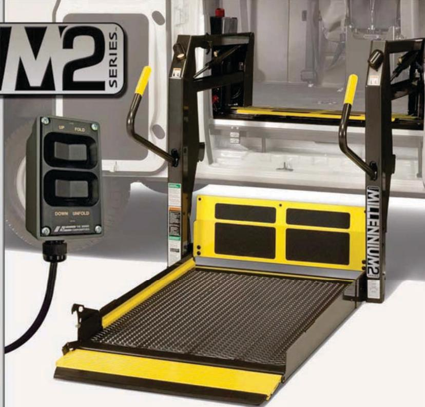
Integrated dual handrails provide added security for wheelchair users and standees
