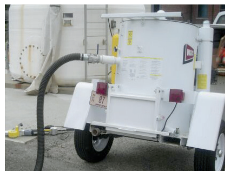
Large capacity holding tank with manually activated dump gate makes emptying simple
