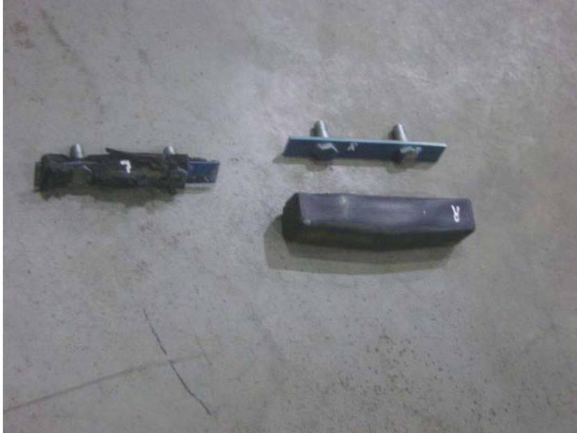
BROKEN FRONT AXLE BUMP STOPS (764 TEST MILES)
