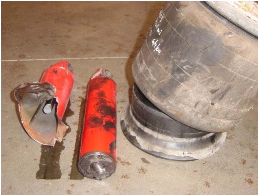
BROKEN SHOCK PUNCTURED AIR BAG (5,571 TEST MILES)
