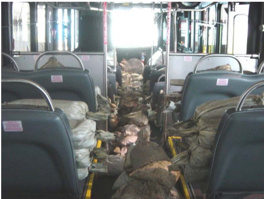
BUS LOADED TO 2.5 TIMES GVL (28,125 LBS)
