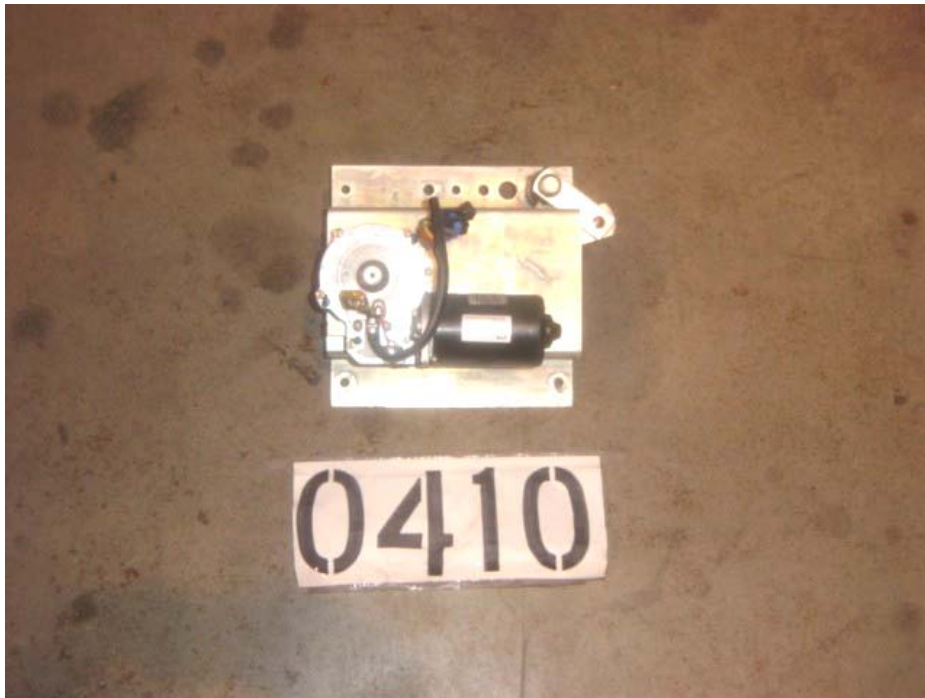
WIPER MOTOR REMOVAL AND REPLACEMENT (0.50 MAN HOURS)
