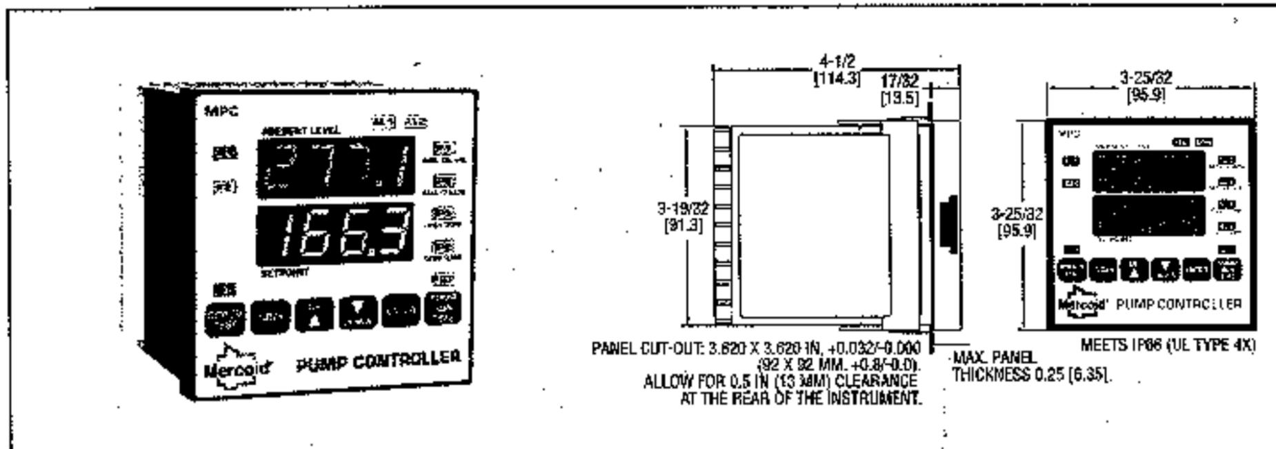
The Mercoïd<sup>®</sup> MPC Pump Controller provides versatile level control in a standard 1/4 DIN package. Designed for use with almost any style level transmitter the unit displays the present level and main set point value. Incorporated in the MPC is programmable level differential for on/off control of one or two pumps, valves, or other devices through two SPDT relays. Also featured are two additional programmable alarm contacts with front status light indication.
