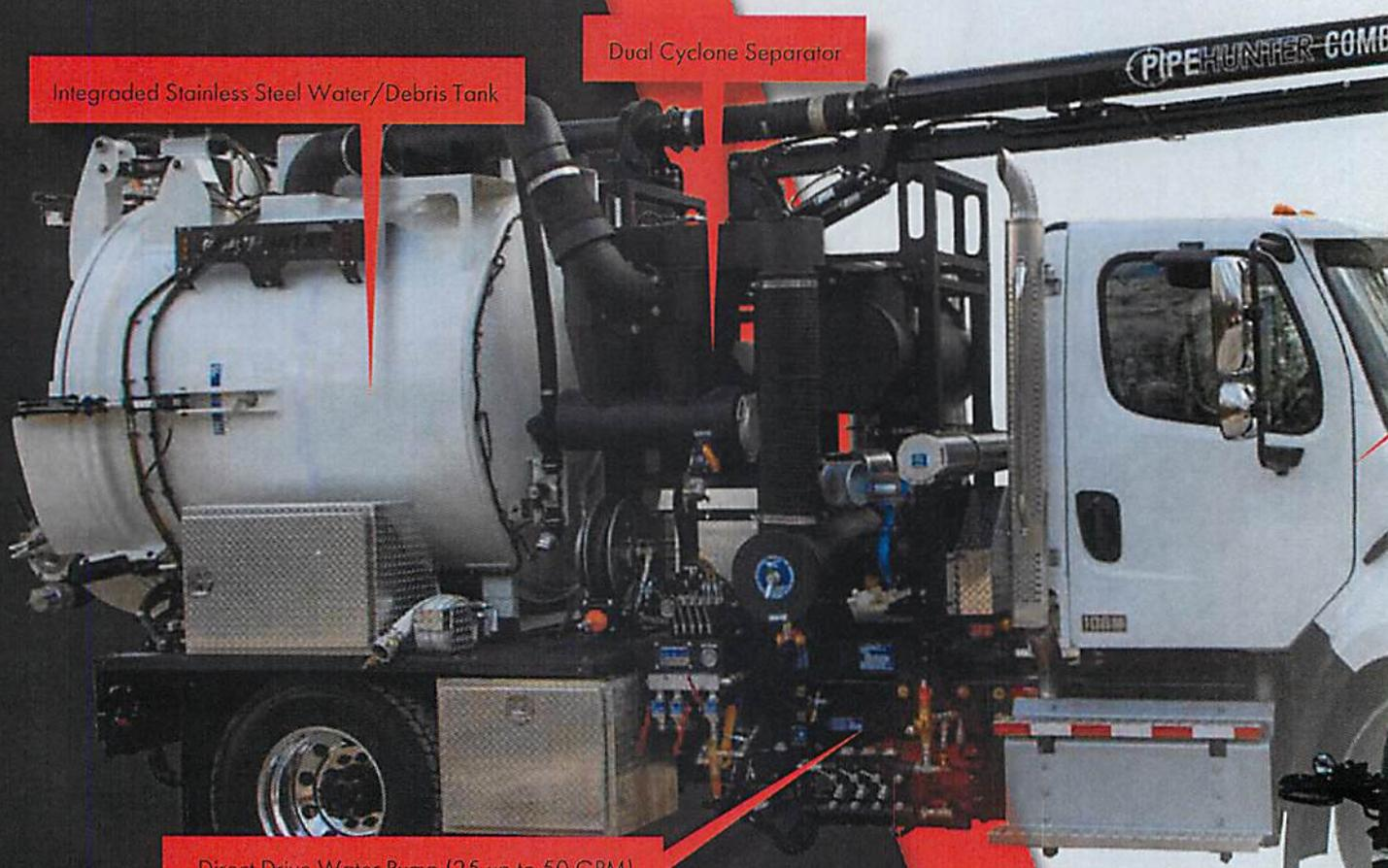
Integrated Stainless Steel Water/Debris Tank
