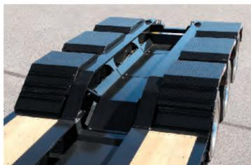
**Knuckle and Boom Troughs, 3rd Lift Axle**
