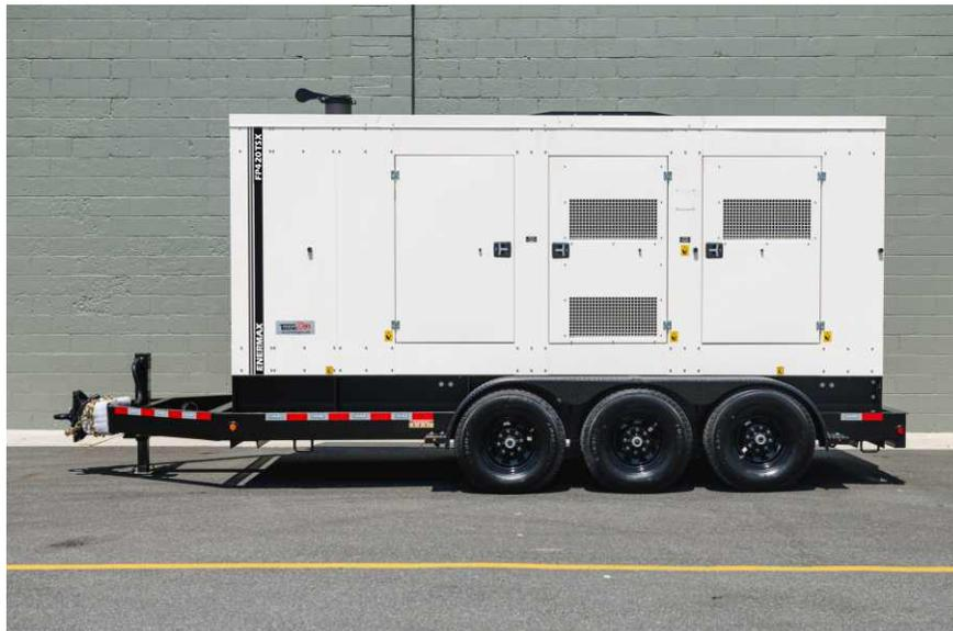
TecnoGen's 420kVA generator uses the FPT engine coupled to an industry standard Leroy Somer alternator producing 334kW of prime power. Standard features include camlocks, block heater and battery charger. The Deep Sea controller makes retrieving vital stats like fuel levels, run time and start logs easy and the sealed doors and 2" thick insulation throughout gives this gen a 70 dBA rating.
