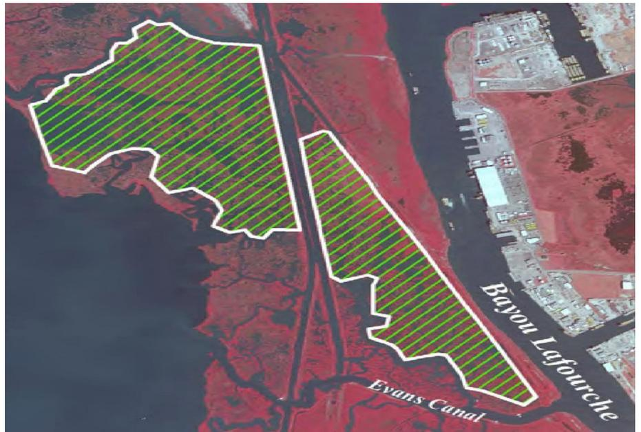
It should be noted that Ardaman has worked with CPRA through GIS and the Port of Fourchon on investigating an alternative borrow source within Bayou Lafourche and adjacent Port slips. The supplemental field investigation was completed in 2021. The engineering has also been completed in regard to channel stability and reanalysis of the West Fourchon Marsh Creation Areas with the alternative borrow source.
