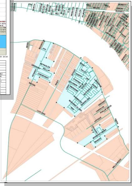
BBEC developed the survey scope of work and managed the surveyor to obtain the needed data for the model. BBEC performed multiple model runs to determine the most cost-effective means to drain the 10-year storm for each subdivision. BBEC developed recommended project scopes and construction cost estimates for each
