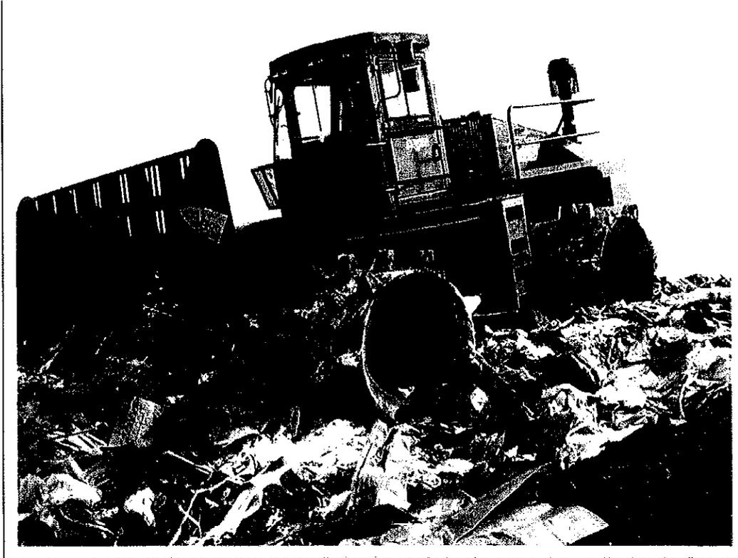
Wheels are 48" wide with 1" thick outer drums, 58" drum diameter and 74" overall diameter measured over the cleats.
