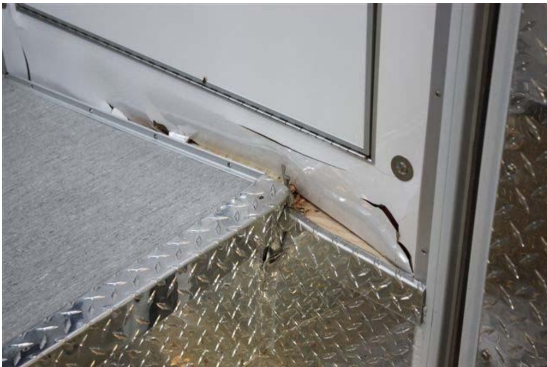
VIEW SHOWING DAMAGE INSIDE PERSONNEL DOOR (TEST 052)
