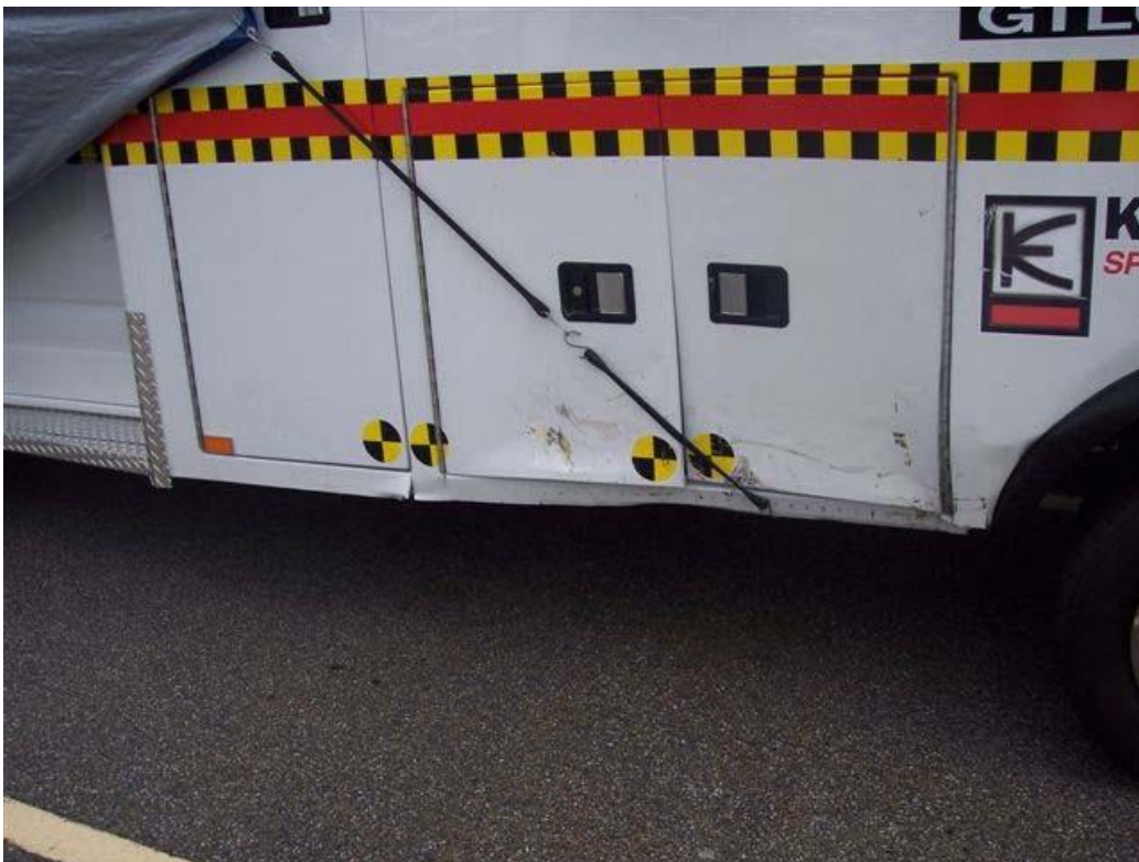
OVERALL VIEW OF LEFT SIDE DAMAGE (TEST #055)
