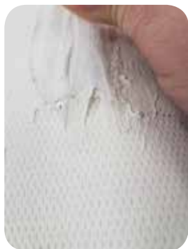
Repair Hero adhesion to aged TPO
