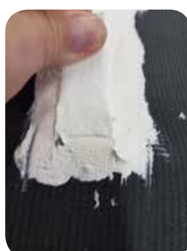
Repair Hero adhesion to aged reinforced EPDM
