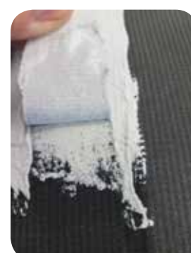
Silicone-based Roof Patch adhesion to aged reinforced EPDM
