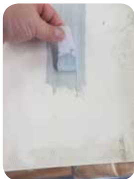
Silicone-based Roof Patch adhesion to aged TPO
